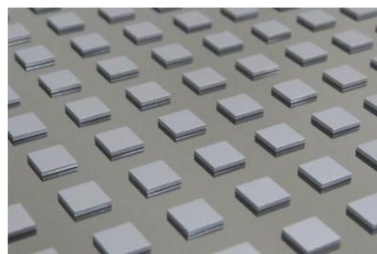
Fig. 10. A photo of an assembled coupon using the EMC/PID system after pre-bonding
