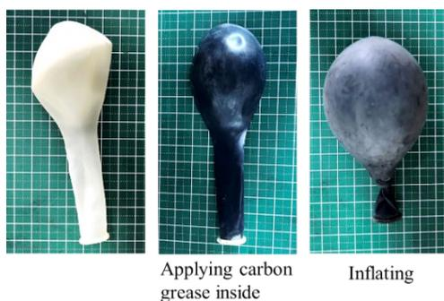
Fig. 2. Actuator creation process
