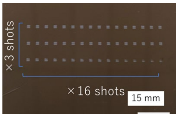
Fig. 9. Photograph of the exposed wafer with the 48 shots.
