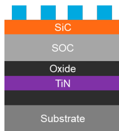
Fig. 4. Stack for AEI in both pillar and L/S patterns.
