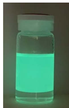
Fig. 6. Photo image of the mixture of reagents for chemiluminescence using betaine 30 as a dye in toluene.
