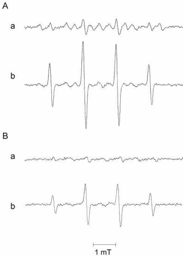
Fig. 5. Hydroxyl radical formation in the reaction of H_2O_2 (a) or D-Pc (b) with urine (A) or Cu-Glu complex (B).
